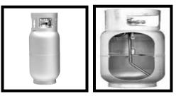
**WARNING:** Using a liquid withdrawal (fork truck) propane tank will clog the orifice in the heat tool and result in an extremely long and dangerous flame.
