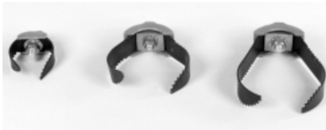
Figure 4 – T-411 2", T-413 3" & T-414 4" Cutter: Used for general cleaning to remove tree roots and materials clinging to pipe walls.
