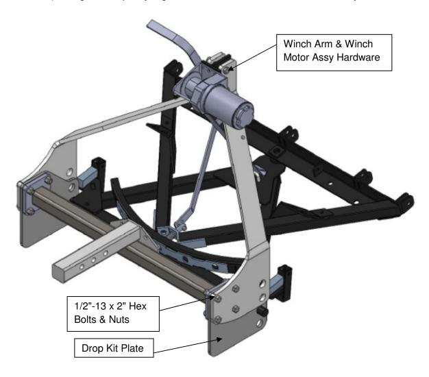
Drop Kit is installed and ready for use.
